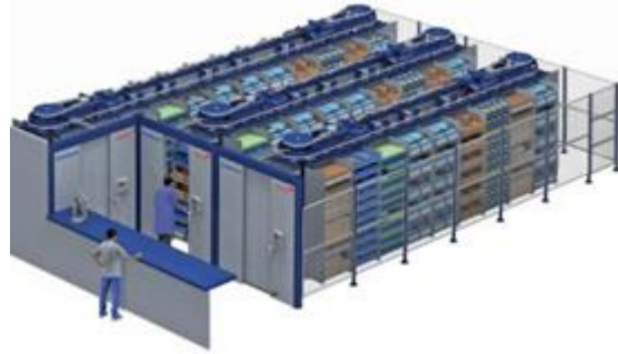
Automated horizontal warehouse
